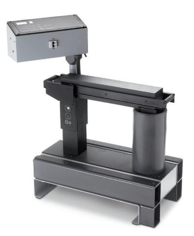
The large simatherm induction heater for roller bearings and other circular metal workpieces up to 850 mm bore diameter and a cross section of 330 x 355 mm. With the integrated time and temperature controls, roller bearings can be heated to the prescribed 110°C while other circular metal workpieces can be heated to 400°C.
