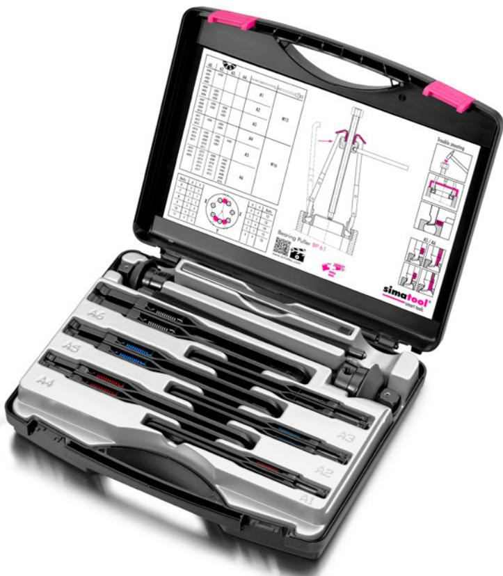
With the extractor tool BP 61, deep groove ball bearings can be removed from the shaft. It is also equally suited for removing bearings from just a shaft. Even sealed bearings can be dismounted once the seal is removed. The hooks of the puller arms are placed in the outer ring. The toolset can be used with 61 different kinds of deep groove ball bearings with diameters of 10 to 100 mm.
