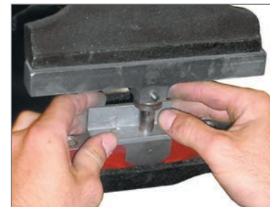
Bench vise used vertically as a press.
