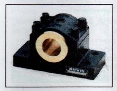
The DIN506 is a heavy duty four bolt plummer block which consists of a fully split cast iron housing and a split gunmetal bush. The units are suitable for grease lubrication and replacement bushes can be easily fitted.
