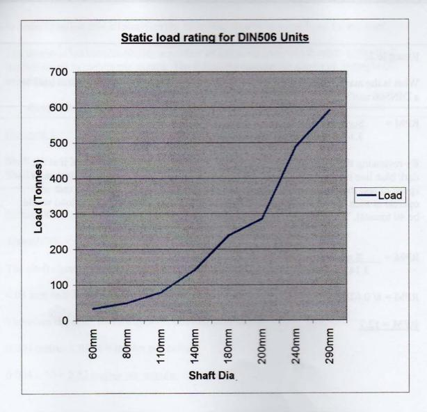
The chart shown above details the static load capacity of DIN506 units.
