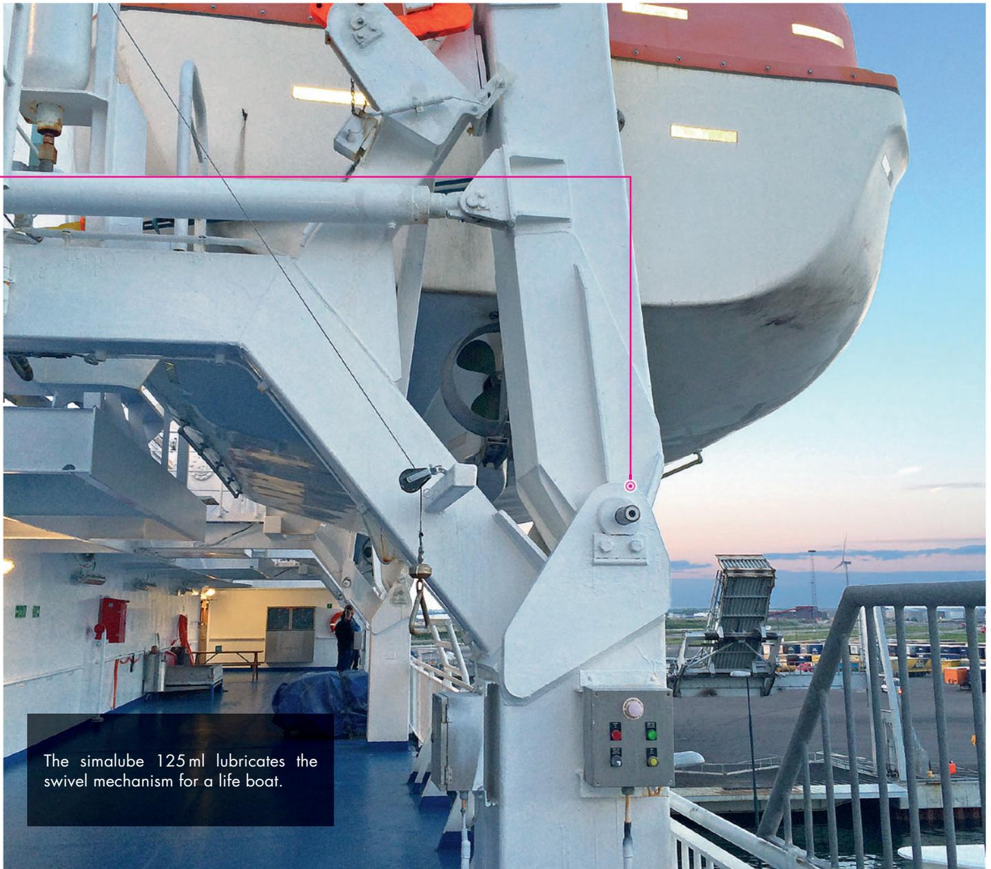
The simalube 125 ml lubricates the swivel mechanism for a life boat.
